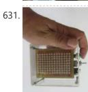
GYRO & VOICE ARDUIGAMES This gaming box is made from Arduino Uno R3, LoLShield, MPU6050 and Microphone module. With LoLShield, we can show a message/scrolling message or animation picture like: plasma effect, sinewave effect... With MPU6050, we can read value from accelerometer and gyroscope to control movement for simple...... Listed under: Game – Entertainment Projects
