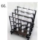
Arduino LED Cube Spectrum Analyzer In this project we'll create a small add-on PCB containing the a MSGEQ7 spectrum analyzer circuit and show how it can drive the RGB LED cube kit from Freetronics. This allows the cube to display the seven bands over four horizontal planes. There is a small amount..... Listed under: LED Projects
