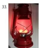
NeoPixel Ancient Oil Lamp In this Instructable, we will describe how to turn a "retro" oil lamp into a NeoPixels based rechargeable lamp with colorful light effects. Supplies Arduino nano12 bits NeoPixel ringMicro USB 5V 1A TP4056 Lithium battery charger module3.7V 9800mAh Lipo Li-polymer BatteryRotary encoder Ec11 or KY-040..... Listed under: Other Projects
