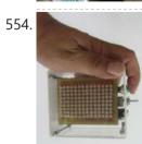
GYRO & VOICE ARDUIGAMES This gaming box is made from Arduino Uno R3, LoLShield, MPU6050 and Microphone module. With LoLShield, we can show a message/scrolling message or animation picture like: plasma effect, sinewave effect...With MPU6050, we can read value from accelerometer and gyroscope to control movement for simple games...... Listed under: Game – Entertainment Projects
