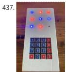
Neo Pixel Tic Tac Toe (Arduino Uno) Tic Tac Toe is a two player game in which the players compete to get 3 pieces in a row. In this project we constructed a Tic Tac Toe game using a number pad and neo pixels as pieces. This results in a portable Tic..... Listed under: <u>LED Projects</u>
