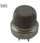
MQ-2 Smoke Sensor Circuit Built with an Arduino In this project, we will go over how to build a smoke sensor circuit with an arduino board. The smoke sensor we will use is the MQ-2. This is a sensor that is not only sensitive to smoke, but also to flammable gas. The MQ-2..... Listed under: Sensor - Transducer - Detector Projects
