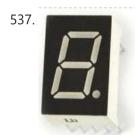
How to Drive a 7 Segment LED Display with an Arduino In this project, we will show how to drive a single 7 segment LED display with an arduino microcontroller. A 7 Segment LED Display is an electronic device housing 8 individual LEDs. Using this device, we can display all numerals and many alphabetical characters and many more...... Listed under: <u>LED Projects</u>
