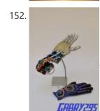
How to Make a Remote Controlled Robotic Hand With Arduino https://youtu.be/efO-ooyS-mo This is my school project for the 5th year of high school (I'm Italian, we have 5 years of high school). It consists in an artificial hand controlled by a glove with flex sensors. The artificial hand reproduces the movements of the hand with..... Listed under: Robotics – Automation Projects
