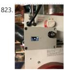
HRV (Home Air Exchanger) Arduino Controller With Air Economizer HRV Arduino Controller with Air Economizer So my history with this project is I live in Minnesota and my circuit board fried on my LifeBreath 155Max HRV. I didn't want to pay the \$200 for a new one. I always wanted something with an air..... Listed under: Home Automation Projects
