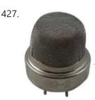
MQ-2 Smoke Sensor Circuit Built with an Arduino In this project, we will go over how to build a smoke sensor circuit with an arduino board. The smoke sensor we will use is the MQ-2. This is a sensor that is not only sensitive to smoke, but also to flammable gas. The MQ-2..... Listed under: Sensor - Transducer - Detector Projects
