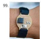
The Nerd Watch Hello! Welcome to another Other Machine project tutorial! I'm Sam DeRose, a former Other Machine Co. Summer Intern. I created the Nerd Watch last summer while working at OMC. The Nerd Watch displays the time in binary when the button is pushed. The watch shows the...... Listed under: Clock – Timer Projects
