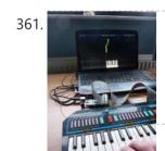
Convert a toy piano to work as a midi device and use it with Synthesia Goal of this project: Convert a cheap toy piano to work as a midi device and use it with Synthesia (http://www.synthesiagame.com/) Other programs that use midi inputs can also be used. Approach: The pushbuttons of the piano are used to make a simple pull-down circuit...... Listed under: <a href="Interfacing(USB - RS232 - I2c - ISP)">Interfacing(USB - RS232 - I2c - ISP)</a> Projects, Sound - Audio Projects
