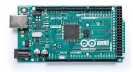
The large number of analog and digital pins, together with a larger memory makes it ideal for devices like 3D printers and other demanding applications.
