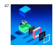
RGB Box Clock https://youtu.be/7inXakX4XOs This is a clock and decorative RGB Led Matrix It's controlled by a Colorduino Shield and NodeMCU v3 Board using i2C communication. With Blynk app you can setup the...
