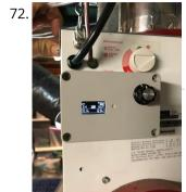
HRV (Home Air Exchanger) Arduino Controller With Air Economizer HRV Arduino Controller with Air Economizer So my history with this project is I live in Minnesota and my circuit board fried on my LifeBreath 155Max HRV. I didn't want...
