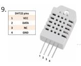
Temperature and Humidity monitoring with DHT22 sensor Arduino Uno R3 The objective of this tutorial is to learn how to use the DHT22 sensor with Arduino uno. The room temperature and humidity will be printed to serial monitor and also...
