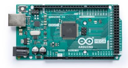
The large number of analog and digital pins, together with a larger memory makes it ideal for devices like 3D printers and other demanding applications.
