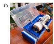
Measuring Refrigerant Gases Sound Speed Using Arduino and App Inventor 2 The purpose of this Instructable is to build a portable device that can measure the speed of sound in refrigerant gases and use this data to identify them. The speed of...
