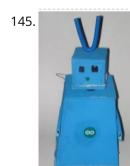
Uno The Arduino Robot Age: 13 Meet Uno the Arduino powered robot. Some functions include a blinking nose, moving antennas, rotating head, IR distance sensor, twin motor gear box and rotation counters. Uno is made with relatively easy to obtain parts. This project provides a good introduction to Arduino. robot.skp475 KB Step 1: Materials Material and tools • Foam board...... Listed under: Projects, Robotics – Automation Projects
