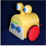
247. Sensor Less 3d Printed Robot Tyree (he wears a tie and he has tires) actually smiles after he bumps into something (see video). Using an Arduino motor shield, he detects obstacles using the "more current into the motor means something is in the way" principle. Tyree started out as a..... Listed under: Robotics – Automation Projects, Sensor – Transducer – Detector Projects
