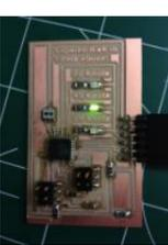
Knockdown Warning Indicator (Redux) This week I continued developing a device that warns of the potential of a knockdown – the process by which an over-canvased sailing ship is lain over on her beam-ends during a squall. The potential for sinking at this point is high, especially if there..... Listed under: Security – Safety Projects, Sensor – Transducer – Detector Projects
