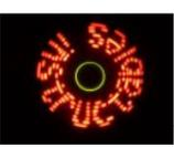
Wooshing leds – Rotated animation by arduino This project allows you draw in the air letters, symbols or other shapes - as you like. Controlled by the Arduino, the 7 simple leds blinking on and off - creating the illusion of floating text in the air. This combination of simple components with..... Listed under: LED Projects
