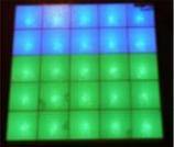
Low Cost LED Grid There are a number of great Instructables on LED grids out there. This is a low cost version - not quite as polished, but easy to make. This project uses a couple of sheets of foam core, a fluorescent fixture cover from the local home..... Listed under: LED Projects
