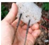
The Soil Moisture Sensor using arduino You are building a cheap soil moisture sensor so the brain can read the amount of moisture in the soil. The version we are building is very low tech, but it is also very cheap and easy to build. It consists of a block of..... Listed under: Home Automation Projects, Temperature Measurement Project Ideas
