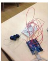
Connect the arduino and make the speaker play To make your Arduino to play a melody you need these accessories. One 5 ohm speaker One Arduino uno board One Push button One 10 kohm resistor 8 leds And a lot of core wires Step 1: Connect the arduino and make the speaker play This..... Listed under: Sound – Audio Projects
