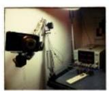
Robot arm from a desk lamp (IKEA Tertial hack) This project answers to a need I had: a third hand that holds a camera while I perform a test and takes photos/videos (useful when you're stuck at the lab late at night, and suddenly need a photographer). The downside to a robotic arm was..... Listed under: Robotics – Automation Projects
