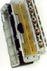
The Photometric Camera and the CCDs The Photometric System The photometric camera for the SDSS consists of two TDI scanning CCD arrays, one, using 30 Tektronix/SITe 2048 x 2048 CCDs in a 5 by 6 array for five-color photometry, and the other using 24 2048 x 400 chips for astrometry and..... Listed under: Video - Camera - Imaging Projects
