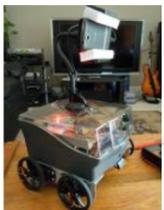
4 Servo drive CellBot which can be remotely controlled using Arduino I started with an idea of what I wanted to do from the beginning but one attempt after another I finally got to where I am now. This robot can be remotely controlled from anywhere in the world and driven around the house. I can..... Listed under: Motor Projects, Projects, Robotics - Automation Projects
