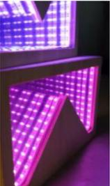
Temperature-Sensitive Infinity Mirro As per an assignment in my digital multi-media class, I've combined two Arduino-related tutorials into a functional object! The result is a pair of infinity mirrors that flash red and blue depending on minute fluctuations in ambient temperature. This is my first experience with Arduino,..... Listed under: Temperature Measurement Projects
