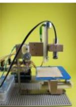
Arduino 3-axis Mini Lazer Paper-Cutter Updated : 16/3 Add step 4, about using the stage. Updated : 18/3 Add photos (cutting vinyl adhesive sheet) Updated : 19/3 Add step 5, acting as pen plotter Updated : 20/3 Add laser engraving video (Wood) and photo Updated : 22/3 Add 2 drawings..... Listed under: Home Automation Projects
