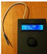
402. Intervalometer for Sony NEX 5n This intervalometer used infrared LED To built intervalometer you need: Arduino Nano (or Arduino-compatibility). I used Nano V3 Serial LCD Joystick Module IR Led and resistor ~200 Ohm Switch Push Button Plastic enclosure Battery 9V Schematic is very simple Step 2: Connection Serial LCD has..... Listed under: Metering – Instrument Projects
