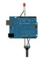
Pulse Width Modulation : PWM using Arduino Pulse Width Modulation or PWM is a method of Digital to Analog Conversion. It helps in delivering analog average voltage using digital pulses of variable pulse width. By controlling the on time and off time, we can generate an analog average voltage using the digital..... Listed under: PWM Projects
