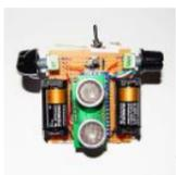
Haptic Proximity Module (HPM) for Low Vision users The Haptic Proximity Module (HPM) seeks to enable people with low vision, or other vision impairments, to engage with their direct surroundings through vibration feedback from a range detector, and do so cheaply with readily available components. The aim of this instructables is to share..... Listed under: Development Board – Kits Projects
