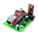
Arduino DDNS (Dynamic DNS) by Open-Electronics.org This device captures the IP address of your network and it publish on site DynDNS.com. All without PC. It allow a remote access to your LAN even if the IP address of the connections changes. For logistics reasons the provider can not assign a IP..... Listed under: Internet - Ethernet - LAN Projects, Projects
