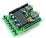
478. A Voice Shield for Arduino Board The objective of this project is to build an Arduino voice shield to empower thousands of voice related applications! All this mostly thanks to an integrated ISD1790PY chip. This particular voice/TTS feature can be useful to integrate voice messages in alarm systems, to implement generic..... Listed under: Projects, Sound - Audio Projects
