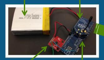
HMC5883 Sensor Arduino Fio
