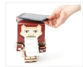
Paper Man is a machine comprised of Arduino, NFC Shield, thermal printer and a papercraft shell—Iron Man. Thanks to the NFC Shield, you can directly sent messages from your mobile...
