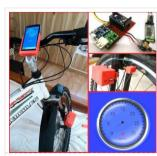
In this project we make a Cool Speedometer for bikes or any automotives by using Arduino which broadcast the speed using Bluetooth to an Android application that we created using Processing. The complete project...
