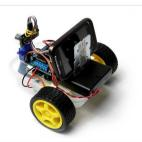
You'll need these: HC-SR04 – Get this ultrasonic sensor from eBay.com.au for \$2. SG90 Servo Motor – We've seen this servo selling for around \$4 on ebay. Motor drive shield...
