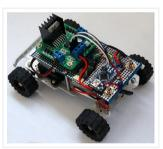
This is a simple project of Android Bluetooth Car with Bluetooth control. Arduino controller is used To control the car used Android-device with a built-in accelerometer. Tilt forward – car goes...
