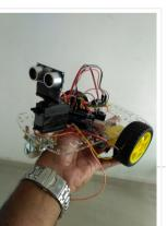
This project is designed to build a robot that automatically detects the obstacle on its path and guides itself whenever an obstacle comes ahead of it. This robotic vehicle is...
