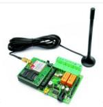
Using an ATmega 2560 and therefore the heart of Arduino, we have developed a universal remote control with GSM. This allows to control 2IN/2OUT, DTMF key, gate control and GSM...
