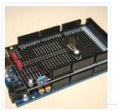
Overview The Arduino Mega 2560 is a microcontroller board based on the ATmega2560 (datasheet). It has 54 digital input/output pins (of which 14 can be used as PWM outputs), 16 analog inputs,...
