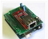
Ethernet Shield description: The Arduino Ethernet Shield allows an Arduino board to connect to the internet. It is based on the Wiznet W5100 ethernet chip. The Wiznet W5100 provides a...
