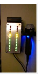
Now with more LED. Arduino mega powered breathalyser using the MQ-3 sensor. A relative gauge for judging how intoxicated you are. NOT TO BE USED AS MEANS OF BREATHALYZING...
